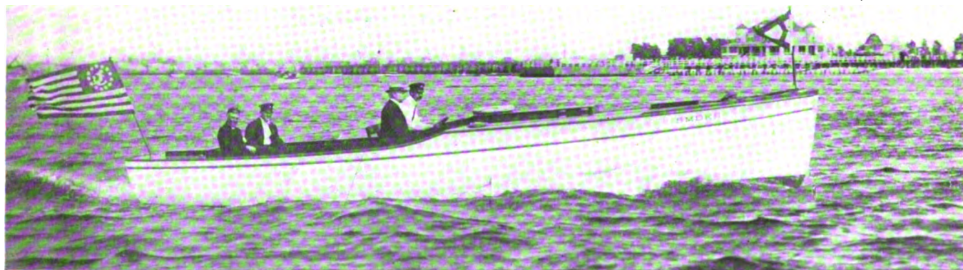
Smoke. Length Over All 32 Ft., Breadth 7 Ft., Draught 2 Ft. 8 In. Power 4-Cylinder 4 \frac{3}{4} In. x 5 \frac{1}{2} In. 20-30-H.P. Sterling Engine. Speed 13 Miles per Hour. Allerton & Brophy, Owners. Designed by John R. Brophy
